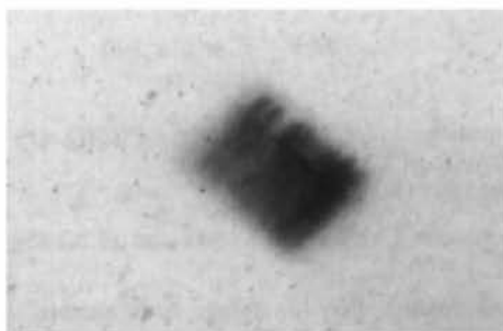
Fig. 1. White-beam X-ray topograph of a lysozyme crystal grown by the hanging-drop method at 288 K and pH 4.7. A few dislocations can be observed in this topograph.
